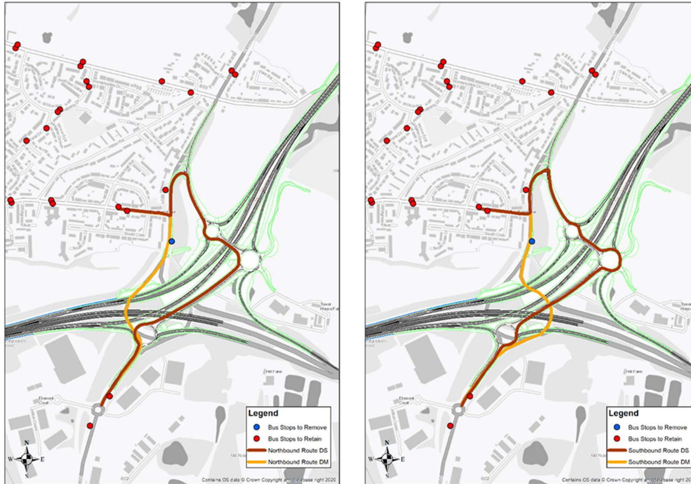
Figure 7.3: Bus Route 70 Northbound (left) And Southbound (right) Through M54 J1 In The DM and DS
